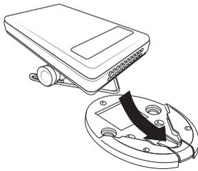
1. Once the unit is assembled and the base mounted, simply snap the wire stand into the base. The latch at the front of the base should snap into place, locking in the stand and unit.
