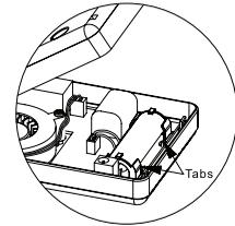
3. Lift the small circuit board holding the target screen and bulb (Bulb Assembly) from the two tabs.
